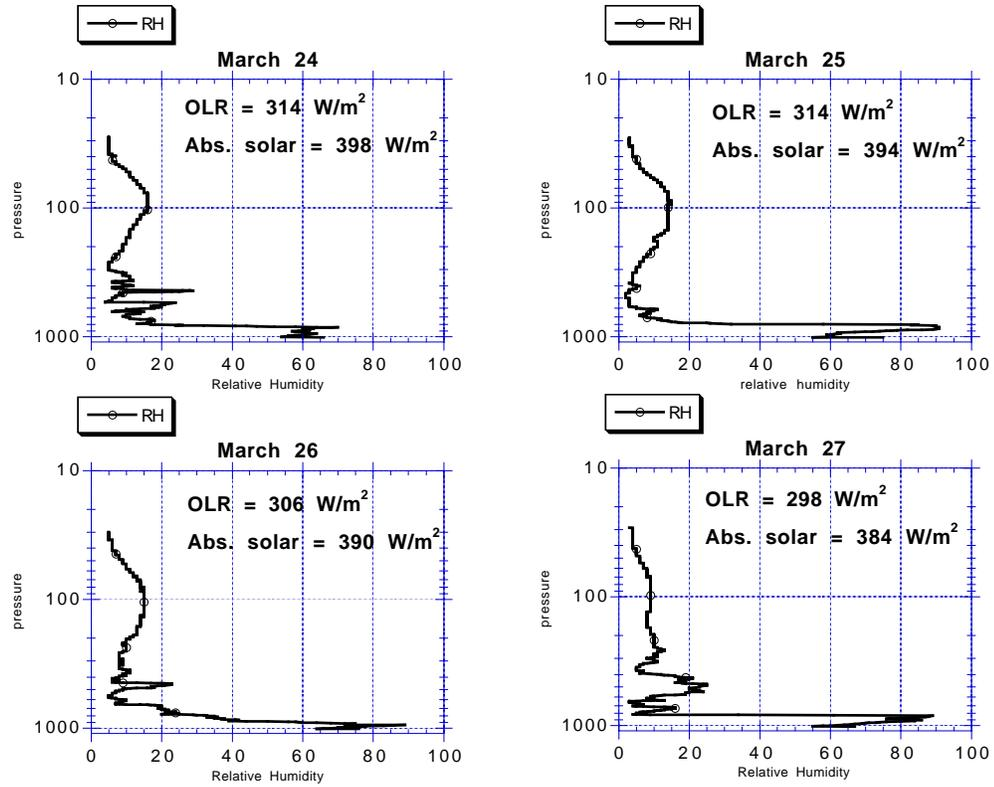
**Figure 2.** Relative humidity profiles of the four subtropical CEPEX soundings. The clear-sky local absorbed solar radiation and outgoing longwave radiation (OLR) were computed for each sounding using a radiative transfer model, and are indicated on the graphs.
