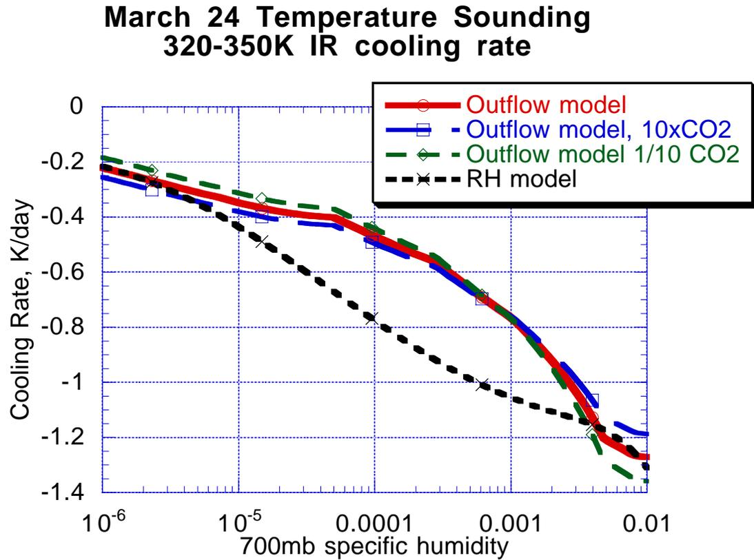
**Figure 3.** Upper tropospheric infrared radiative cooling for the March 24 temperature sounding, as a function of humidity. Results are shown for the RH model and the outflow model. For the outflow model, the cooling is computed also with 10 times present  $CO_2$  and 1/10 present  $CO_2$ . The cooling is averaged over the isentropic layer 320K-350K (about 700-100mb).
