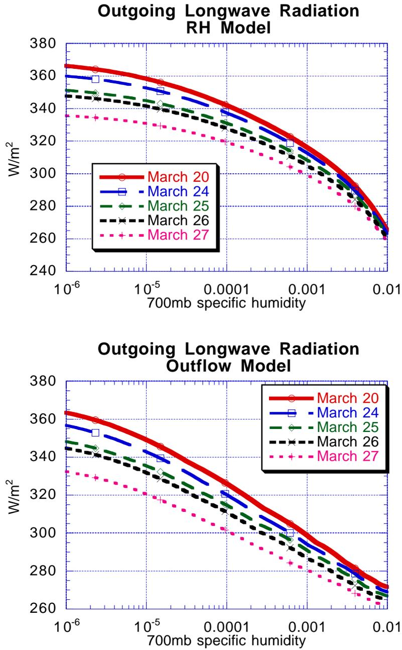
**Figure 5.** Outgoing longwave radiation as a function of 700mb specific humidity for 5 tropical temperature sounding. Results are shown for the RH model (a) and the outflow model (b).
