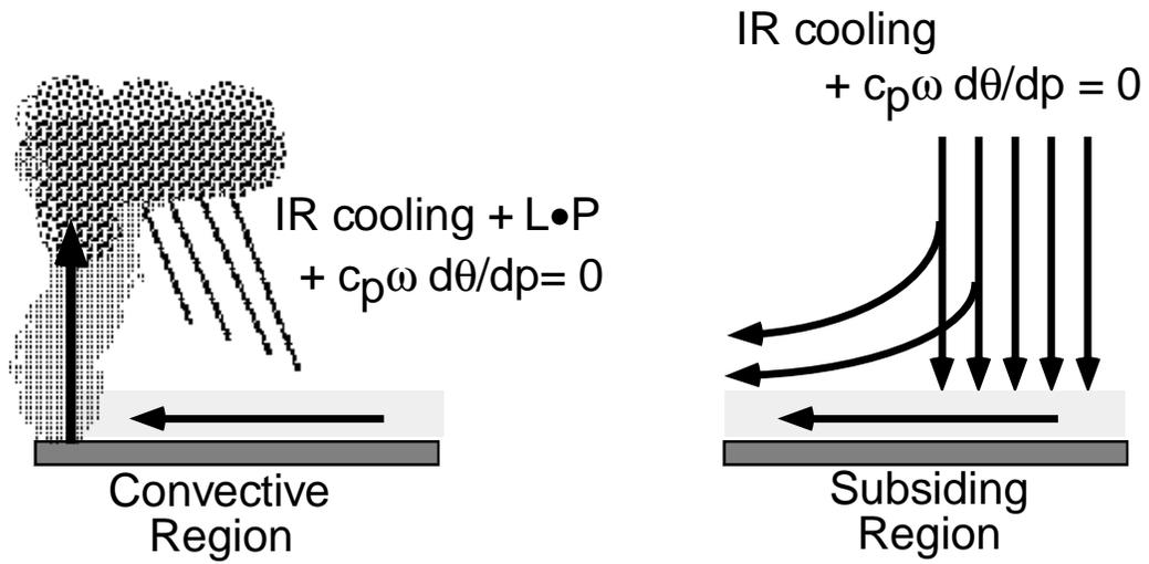
**Figure 4.** Schematic of radiative/dynamic balance in the convective vs. nonconvective region of the Tropics. In this figure  $L$  is the latent heat of condensation,  $P$  is the precipitation rate,  $\omega$  is the pressure velocity and  $\theta$  is the dry potential temperature.
