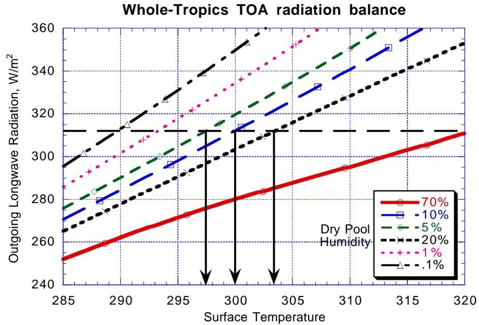
**Figure 6.** Outgoing longwave radiation averaged over the whole tropics, as a function of surface temperature. Curves are computed for various dry-pool humidities. The vertical profile of humidity was taken according to the RH model. See text for details of the calculation.
