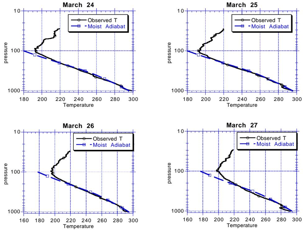
**Figure 1.** Temperature profiles of the four subtropical CEPEX soundings, compared to the moist adiabat.
