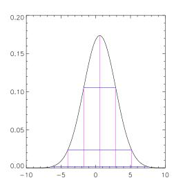
The most complete information you could give is a *Probability Distribution Function* (*PDF*) of the result of an experiment, giving the probability that the result lies in any range. For the three marked ranges( $\pm 1$ ,  $\pm 2$ ,  $\pm 3$  standard deviations) about the mean, the probability is the area between the ordinates (68%,95%,99.7% for this *normal distribution*.)
