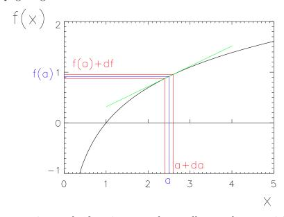
Provided we can approximate the function over the small range by a straight line then it appears from the diagram that  $\sigma_f = \left(\frac{df}{dx}\Big|_a\right)\sigma_a$ .
