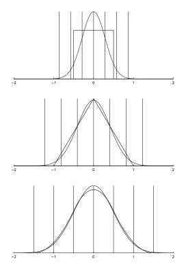
The normal distribution is an important case because of the *central limit theorem*: the PDF of the result of an experiment approaches a normal distribution as the number of different error contributions increases.
