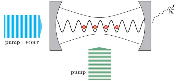
**Fig. 1.** (Color online) Scheme of atoms inside an optical cavity, driven by two external pumping lasers. An additional conservative lattice potential, independent of the intracavity field, is realized by a far off-resonant dipole trap (FORT).
