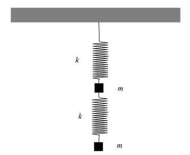
Two equal masses m are connected as shown with two identical massless springs, of spring constant k. Considering only motion in the vertical direction, obtain the differential equations for the displacements of the two masses from their equilibrium positions. Show that the angular frequencies of the normal modes are given by
