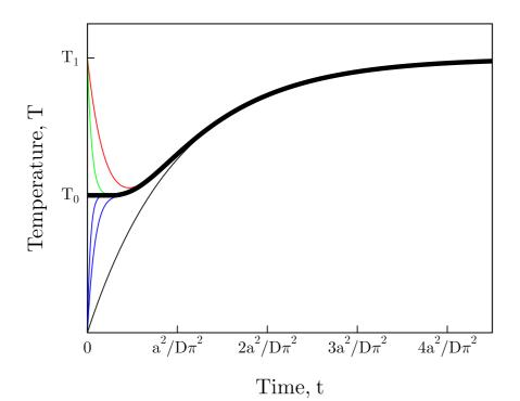
The sum of the first few terms of  $T(0,t) = T_1 + 2(T_1 - T_0) \sum_{n=1}^{\infty} (-1)^n e^{-D(n\pi/a)^2 t}$ are shown, together with T(0,t) evaluated from all terms (thick solid line). The sums of only the first few terms fail near t = 0 and one needs more and more terms to give an accurate estimate of the temperatures as t gets closer to 0 (although this is the region where one knows what the temperature is anyway!)
