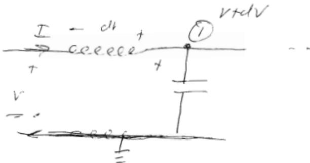
At node 1 There is a current which is through the capacitor that joins  $I$  at location  $Z + dZ$
