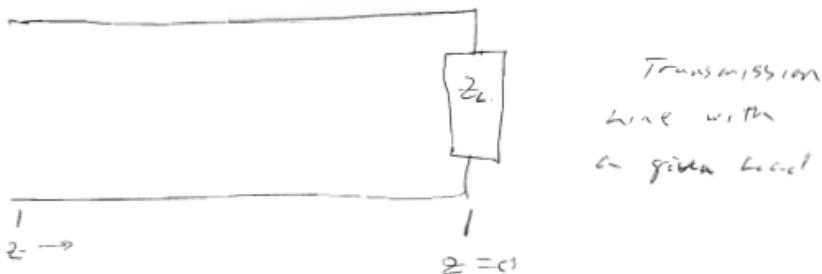
What happens when such a voltage or current wave encounters a terminating impedance?
