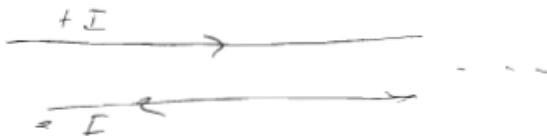
naive view is that  $R_s$  is a wire with zero resistance so the signal travels perfectly with no distortion!
