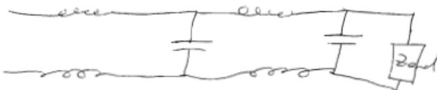
note that  $Z_{\text{end}}$  is in parallel with  $C$
