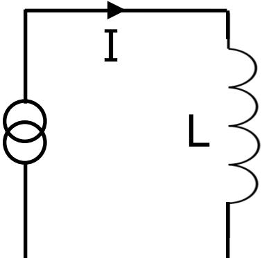
$$V_L = L \frac{dI}{dt} = \omega L I_0 \cos(\omega t) = \omega L I_0 \sin\left(\omega t + \frac{\pi}{2}\right)$$
