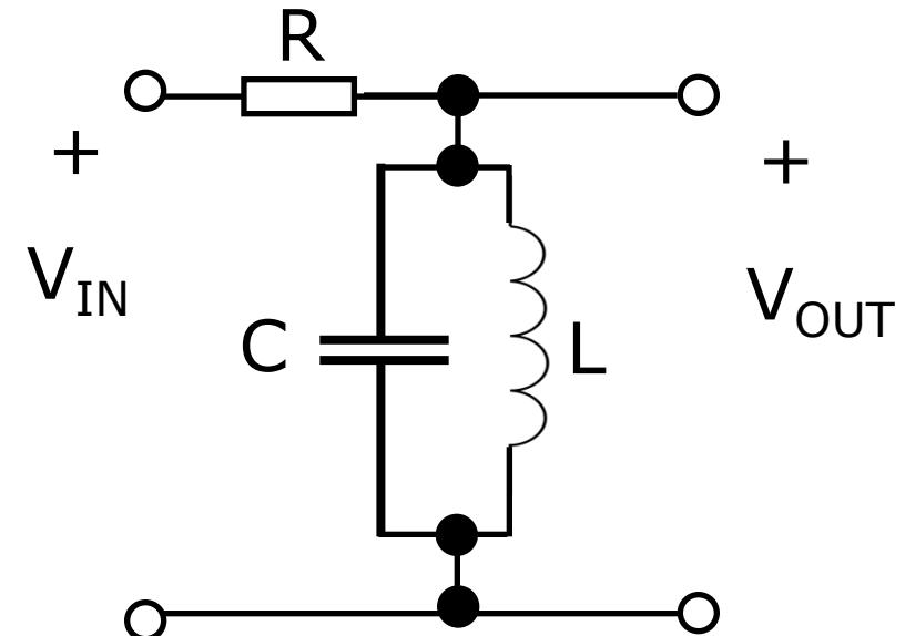
$$\left| \frac{V_{OUT}}{V_{IN}} \right| = \frac{1}{\sqrt{1 + R^2 \left( \frac{1}{\omega L} - \omega C \right)^2}}$$
