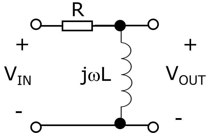
$$V_{OUT} = V_{IN} \frac{j\omega L}{R + j\omega L}$$
