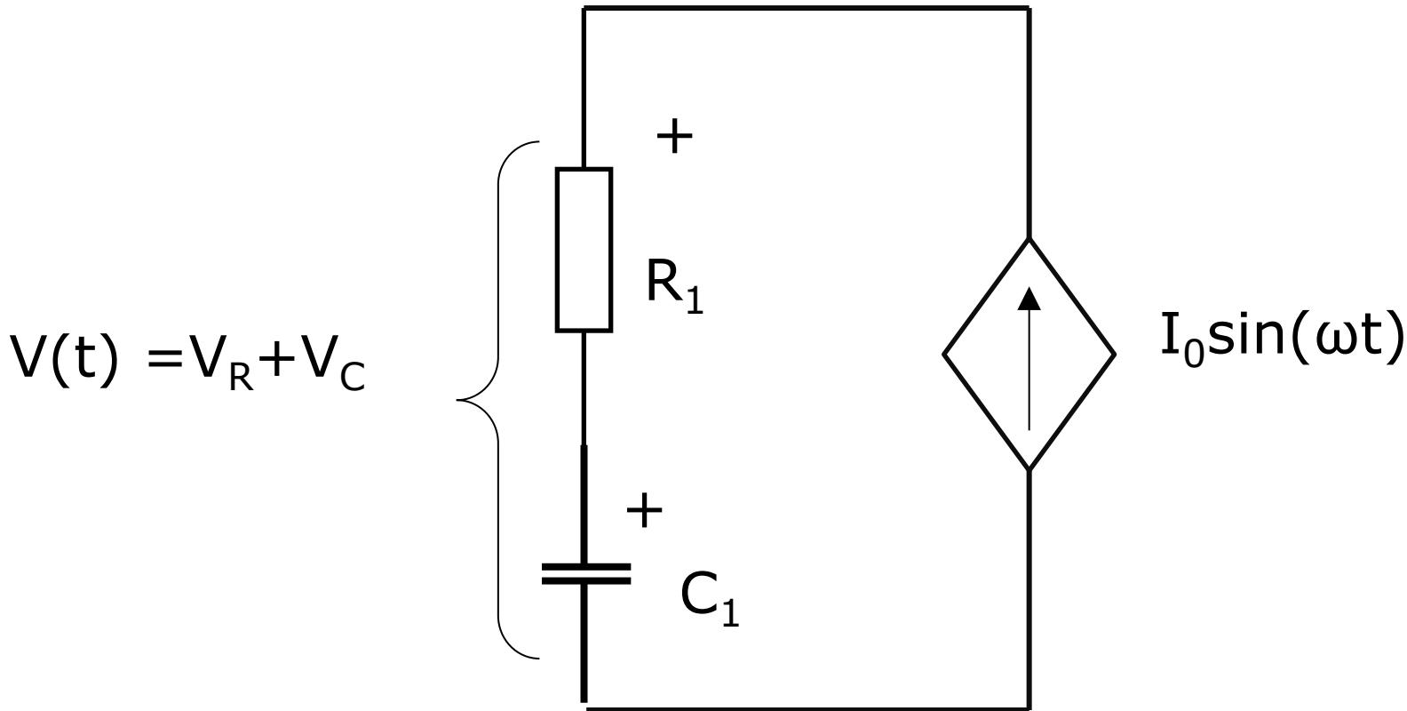
$$V = I_0 R_1 \sin(\omega t) - \frac{I_0}{\omega C} \cos(\omega t) \quad \text{voltages out of phase... } 4$$
