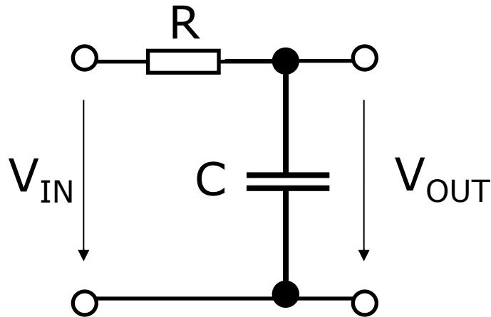
$$\left| \frac{V_{OUT}}{V_{IN}} \right| = \frac{1}{\omega C} \frac{1}{\sqrt{R^2 + \left(\frac{1}{\omega C}\right)^2}}$$
