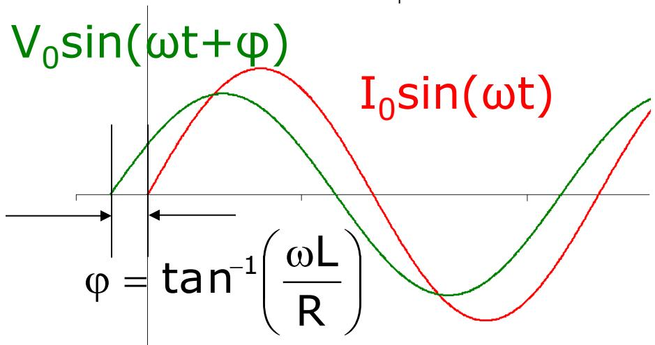
$$V_0 = I_0 \sqrt{R^2 + (\omega L)^2}$$
