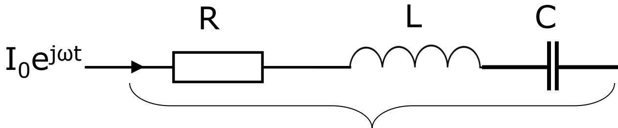
$$\begin{aligned}V &= V_R + V_L + V_C \\&= (Z_R + Z_L + Z_C)I \\&= \left( R + j\left( \omega L - \frac{1}{\omega C} \right) \right) I\end{aligned}$$
