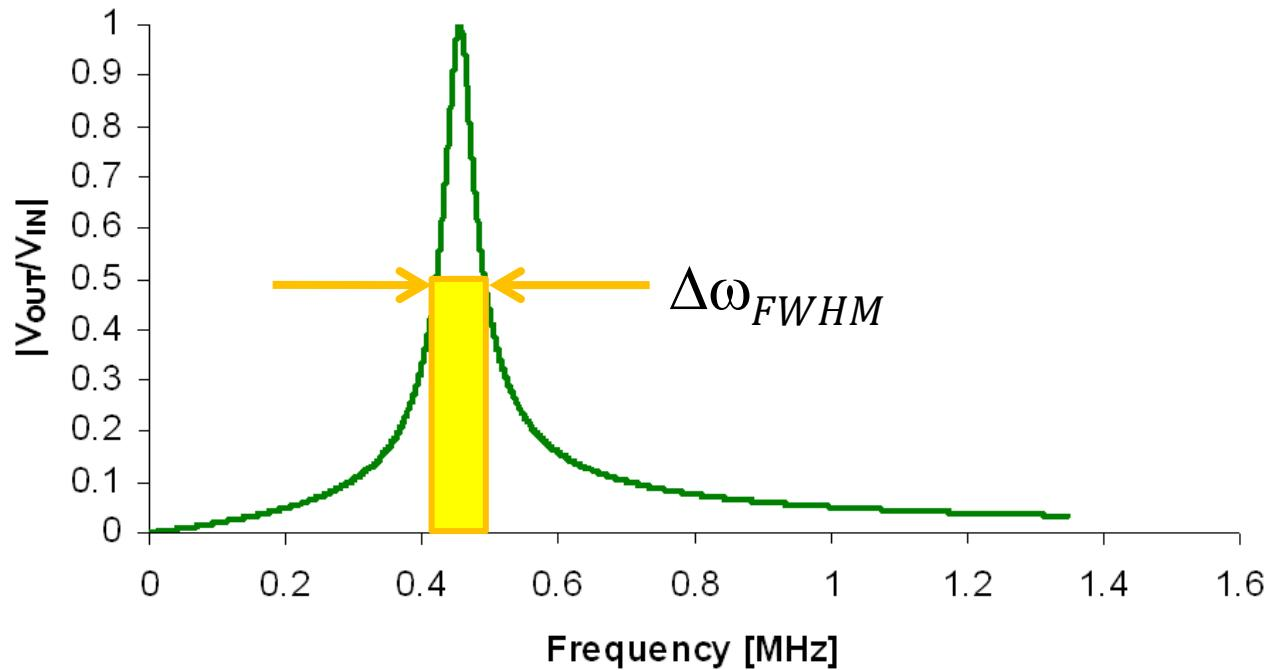
$$Q = \frac{\omega_0}{\Delta\omega_{FWHM}} = \frac{\omega_0}{2\Delta\omega} = \frac{1}{2} \cdot 2R \sqrt{\frac{C}{L}} = R \sqrt{\frac{C}{L}}$$
