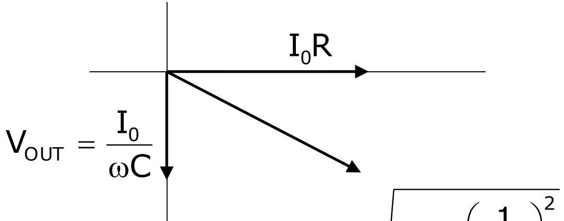
$$\omega \rightarrow \infty \quad \left| \frac{V_{OUT}}{V_{IN}} \right| \rightarrow 0$$
