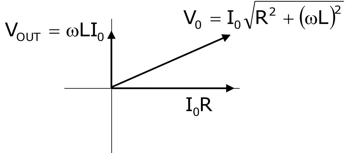
$$\left| \frac{V_{OUT}}{V_{IN}} \right| = \omega L \frac{1}{\sqrt{R^2 + (\omega L)^2}}$$
