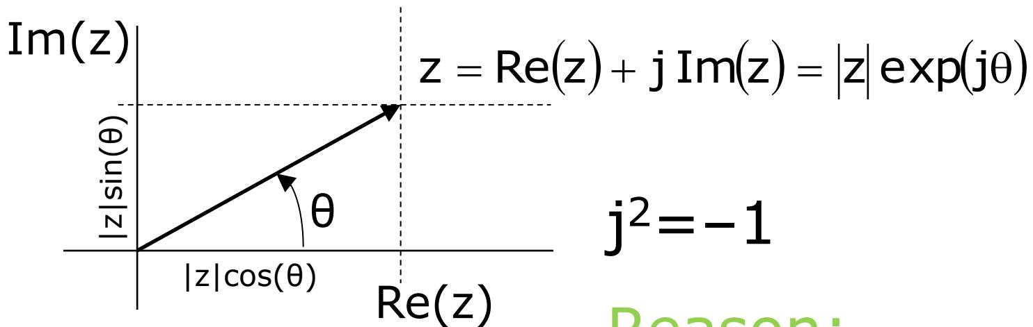
$$V(t) = V_0 \cos(\omega t) = \mathcal{R}e(V_0 e^{j\omega t})$$
