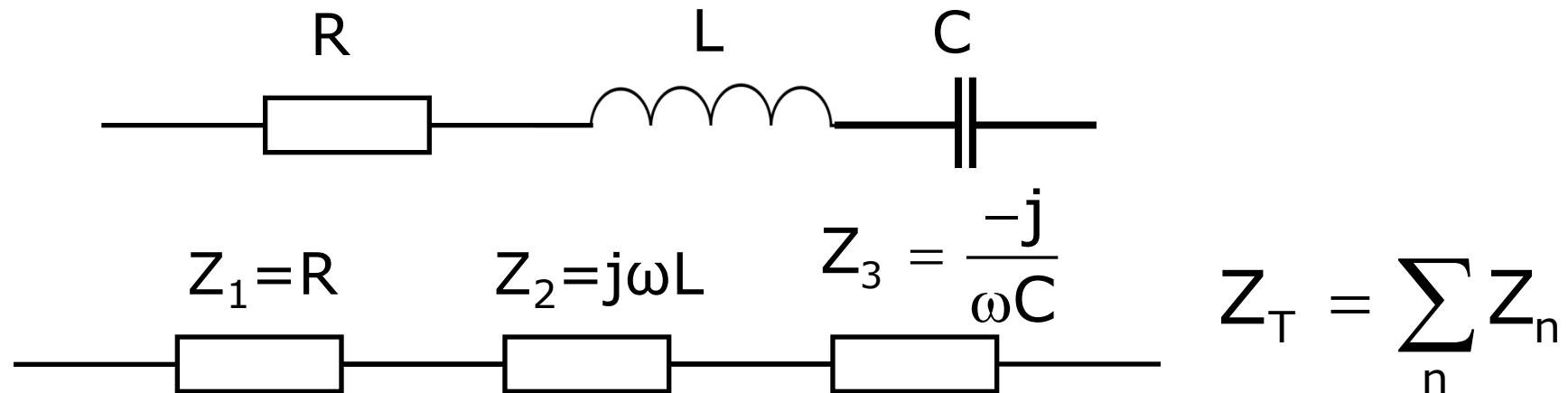
Impedances in series:  $Z_{\text{Total}} = Z_1 + Z_2 + Z_3 \dots$
