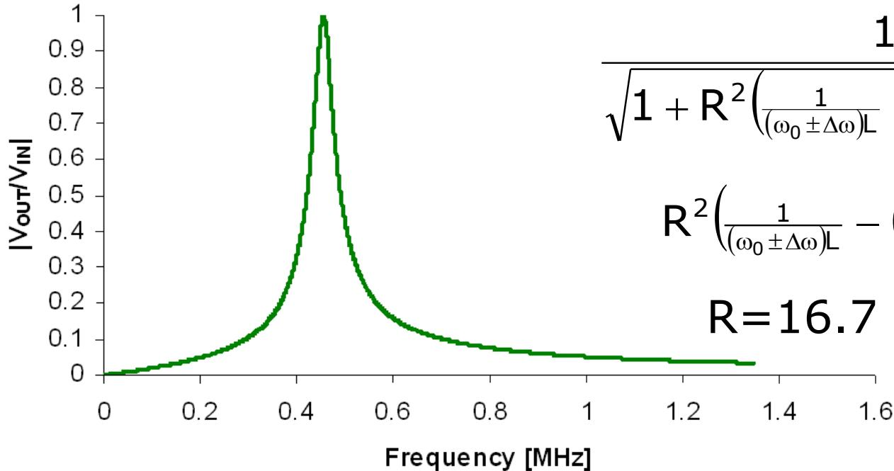
$$\frac{1}{\sqrt{1 + R^2 \left( \frac{1}{(\omega_0 \pm \Delta\omega)L} - (\omega_0 \pm \Delta\omega)C \right)^2}} = \frac{1}{\sqrt{2}}$$
