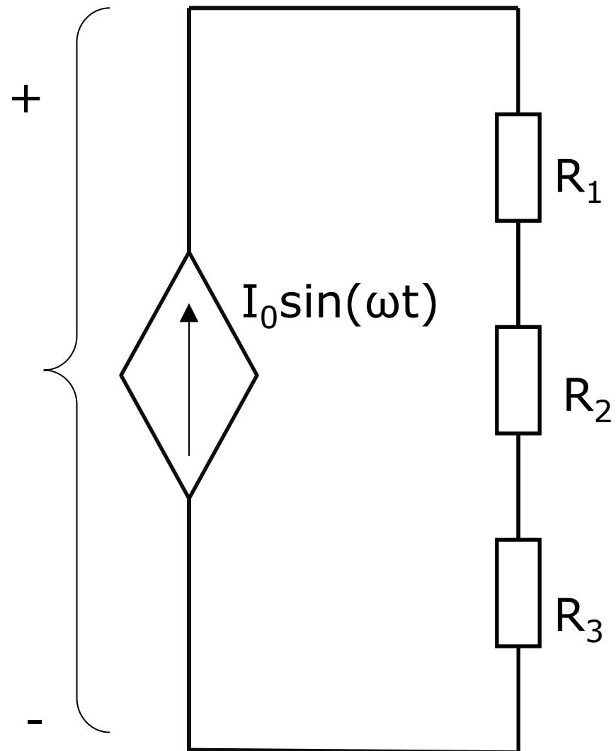
$$\begin{aligned}V &= I_0 R_1 \sin(\omega t) + I_0 R_2 \sin(\omega t) + I_0 R_3 \sin(\omega t) \\&= I_0 (R_1 + R_2 + R_3) \sin(\omega t)\end{aligned}$$
