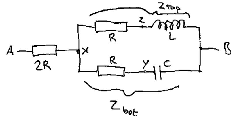
$$V_{xA} = \frac{2R}{Z_{AB}} V_{AB} = \frac{1}{5} V_{AB}$$
