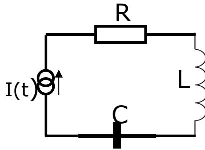
Power is only dissipated in the resistor
