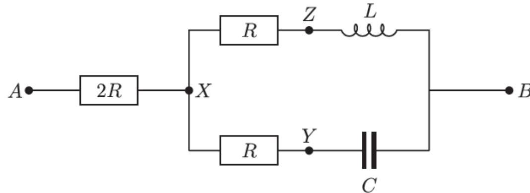
A voltage  $V_{AB} = V_0 \cos \omega t$ , where  $V_0$  is a real amplitude, is applied between the points A and B in the network shown. Given that  $\omega C = 1/(R\sqrt{15})$  and  $\omega L = R\sqrt{15}$ ,
