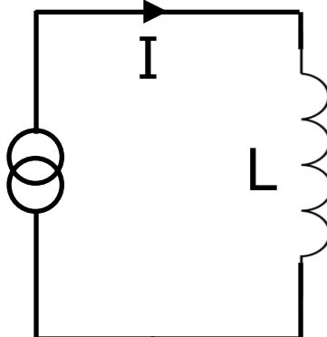
$$V_L = L \frac{dI}{dt} = \omega L I_0 \cos(\omega t) = \omega L I_0 \sin\left(\omega t + \frac{\pi}{2}\right)$$
