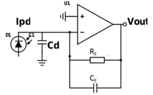
Calculate the feedback factor  $\beta$  and hence explain how this circuit can be tuned to avoid the problem with oscillations.
