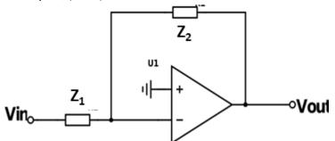
(b) Consider an OpAmp with an open loop gain which varies with frequency as  $A_{OL} = A_0 / (1+j\omega/\omega_c)$ , with A0=10^6 and fc= $\omega_c / (2\pi)$ =10 Hz.
