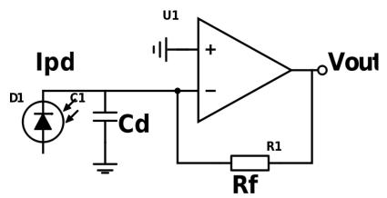
The stability of the transimpedance amplifier can be improved by the addition of a small feedback capacitor in parallel with the feedback resistors as shown in the figure below.
