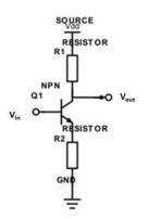
4. Potentiometer biasing for common emitter configuration. Consider the circuit shown below. We want to bias the transistor to be in the active region, so we can assume  $V_{be}$ =0.6V.
