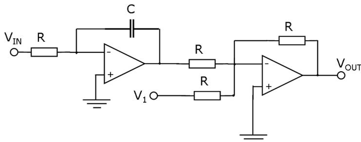
25. For the circuit below, calculate the ratio  $\left| \frac{V_{OUT}}{V_{IN}} \right|$  as a function of  $R$ ,  $C$  and the angular frequency  $\omega$ . At what frequency does  $\left| \frac{V_{OUT}}{V_{IN}} \right| = \frac{1}{\sqrt{2}}$ ? What are the benefits of an active filter such as this, over a simple RC filter?
