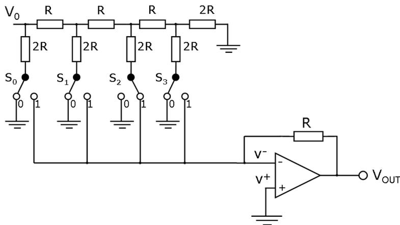
When  $V_0=10V$ , what is the range of  $V_{OUT}$ ? Design a simple circuit to rescale the output to the range 0 to +5V
