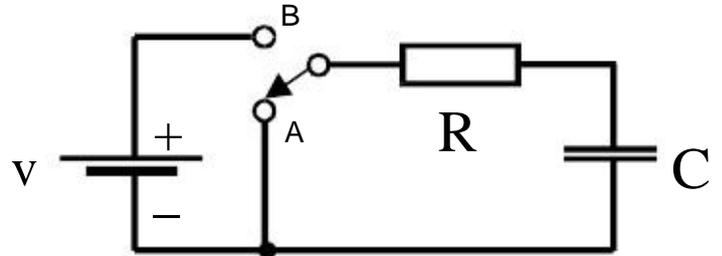
9. Initially the switch in the circuit below is open and the capacitor is uncharged. At time  $t=0$  the switch is closed. Show that the voltage  $V_C(t)$  across the capacitor as a function of time goes as:
