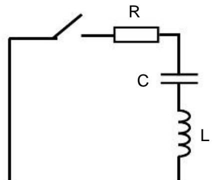
12. In the RLC circuit shown, at time  $t=0$  the switch is closed. By solving the appropriate differential equation, show that the voltage  $V_{out}$  is oscillatory and damped with an exponential decay-time constant given by  $t_0=2CR$ . If the component values are  $R=100\text{ k}\Omega$ ,  $C=0.01\text{ }\mu\text{F}$  and  $L=4\text{ mH}$ , show that the resonant frequency,  $\omega_0$ , is equal to  $1.6\times 10^5\text{ rad/s}$ .
