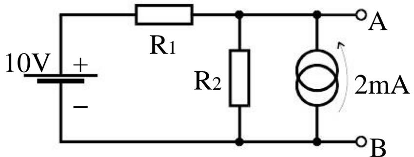
Find the voltage between A and B and the currents  $I_1$  and  $I_2$  through the resistors  $R_1$  and  $R_2$ . Considering Thevenin's theorem, what are  $V_{eq}$  and  $R_{eq}$  in the equivalent circuit? What is the equivalent circuit according to Norton's theorem? Find  $I_{eq}$  and  $R_{eq}$  in this case.
