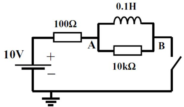
After many time constants have elapsed, the switch is again closed. Show that the voltage across the  $100\Omega$  resistor rises exponentially with time with a time constant of  $1\text{ ms}$ .
