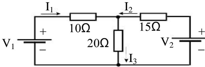
Given  $V_1=5V$  and  $V_2=10V$ , find  $I_1$ ,  $I_2$  and  $I_3$ . Hint: you may wish to tackle the problem using mesh currents.
