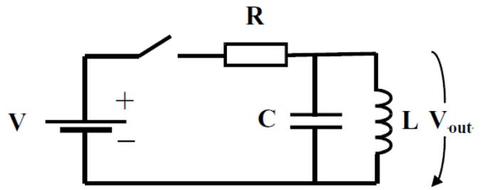
13. The switch in the figure has been closed for a long time, ie. a steady state has been reached, it is then suddenly opened. Demonstrate that  $V_A = V_B = 0\text{V}$  before the switch is opened,  $V_A = 10\text{V}$ ,  $V_B = 1010\text{V}$  immediately after the switch is opened, then that  $V_B$  falls exponentially to  $10\text{V}$  with a time constant of  $10^{-5}\text{s}$
