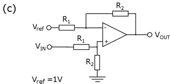
24. For the circuit below, calculate  $V_{OUT}$  as a function of time for an input voltage of  $V_{IN} = \begin{cases} 0 & t < 0 \\ 1V & t \geq 0 \end{cases}$
