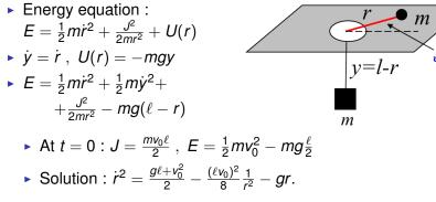
Condition for the particle on the table to move in circular motion  $\rightarrow \dot{r} = 0$ , Equate forces  $\frac{mv_0^2}{\ell/2} = mg \rightarrow \text{gives} \quad \frac{v_0^2}{\sigma\ell} = \frac{1}{2}$
