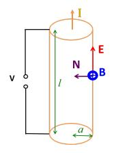
► Total power dissipated in wire :  $P = \int_{S} \mathbf{N} \cdot d\mathbf{a} = VI$  as expected from circuit theory.
