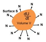
Poynting vector  $\underline{\mathbf{N}}$  is the power per unit area flowing through the surface bounded by volume  $\mathcal{V}$ . (It also gives the direction of flow). Units of  $\underline{\mathbf{N}}$ :  $[W m^{-2}]$
