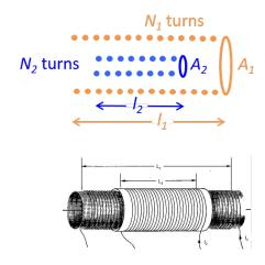
In general circuits may not be tightly coupled, hence  $M = k\sqrt{(L_1 L_2)}$  where k < 1. k is the *coefficient of coupling*.
