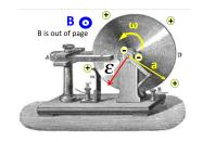
\* Strictly speaking, this method from Faraday's Law is not entirely sensible since the current is continuous across the disk and  $\int_S \underline{\mathbf{B}} \cdot \underline{\mathbf{da}}$  is in principle only applicable for a surface bounding a closed current path (see for example Griffiths).
