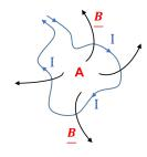
Faraday: The changing magnetic flux  $\Phi$  induces an EMF (voltage) in the loop *itself*:
