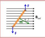
Torque on a magnetic dipole in an external magnetic field  $\mathbf{B}_{\text{ext}}$ :
