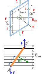
(\*) This has been done for a rectangular shape. But note that this is a general result for *any* shape. Any current loop can be built from infinitesimal rectangular loops with all the internal currents cancelling, yet contributing to the overall moment.
