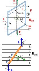
(\*) This has been done for a rectangular shape. But note that this is a general result for *any* shape. Any current loop can be built from infinitesimal rectangular loops with all the internal currents cancelling, yet contributing to the overall moment.
