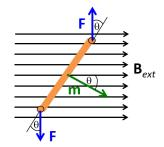
Compare with the energy of an electric dipole  $W_{elec} = -\underline{\mathbf{p}} \cdot \underline{\mathbf{E}}_{ext}$
