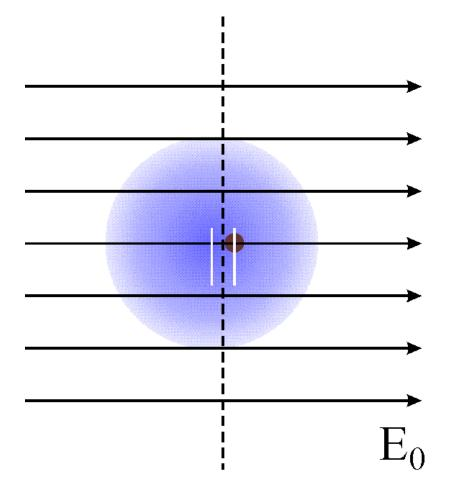
Centres of gravity of the positive nucleus and the negative electron charge distribution shift.
