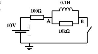
After many time constants have elapsed, the switch is again closed. Show that the voltage across the  $100\Omega$  resistor rises exponentially with time with a time constant of 1 ms.
