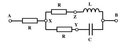
i) Show that the total impedance between A and B is 3R; ii) Verify that voltages of equal amplitude are developed between the points X-A, the points X-Y and the points X-Z; iii) Show that the phases of these three voltages relative to  $V_{AB}$  are 0,  $+\sqrt{3}$  and  $-\sqrt{3}$ .
