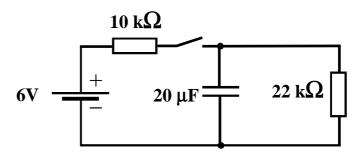
When the steady state has been reached, what is i) the power dissipated in each resistor and ii) the energy stored in the capacitor ?
