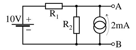
Find the voltage between A and B and the currents  $I_1$  and  $I_2$  through the resistors  $R_1$  and  $R_2$ . Considering Thevenin's theorem, what are  $V_{eq}$  and  $R_{eq}$  in the equivalent circuit? What is the equivalent circuit according to Norton's theorem? Find  $I_{eq}$  and  $R_{eq}$  in this case.
