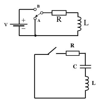
12. In the circuit of question 11, by making any necessary approximations (i.e. verify very light damping), calculate the energy dissipated in the circuit over a cycle, the energy stored in the circuit for the same cycle, and hence show that the Q- value of the circuit has a value of 6.7.
