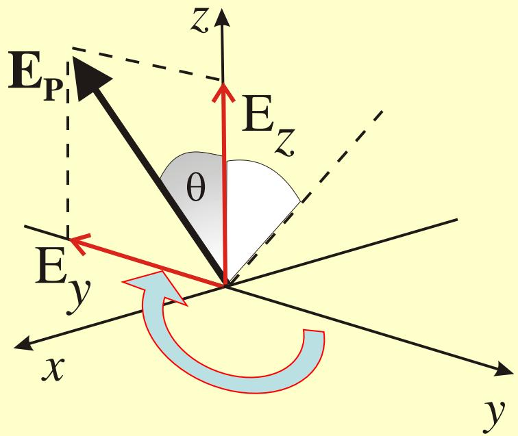
Half-wave plate: introduces  $\pi$ -phase shift
