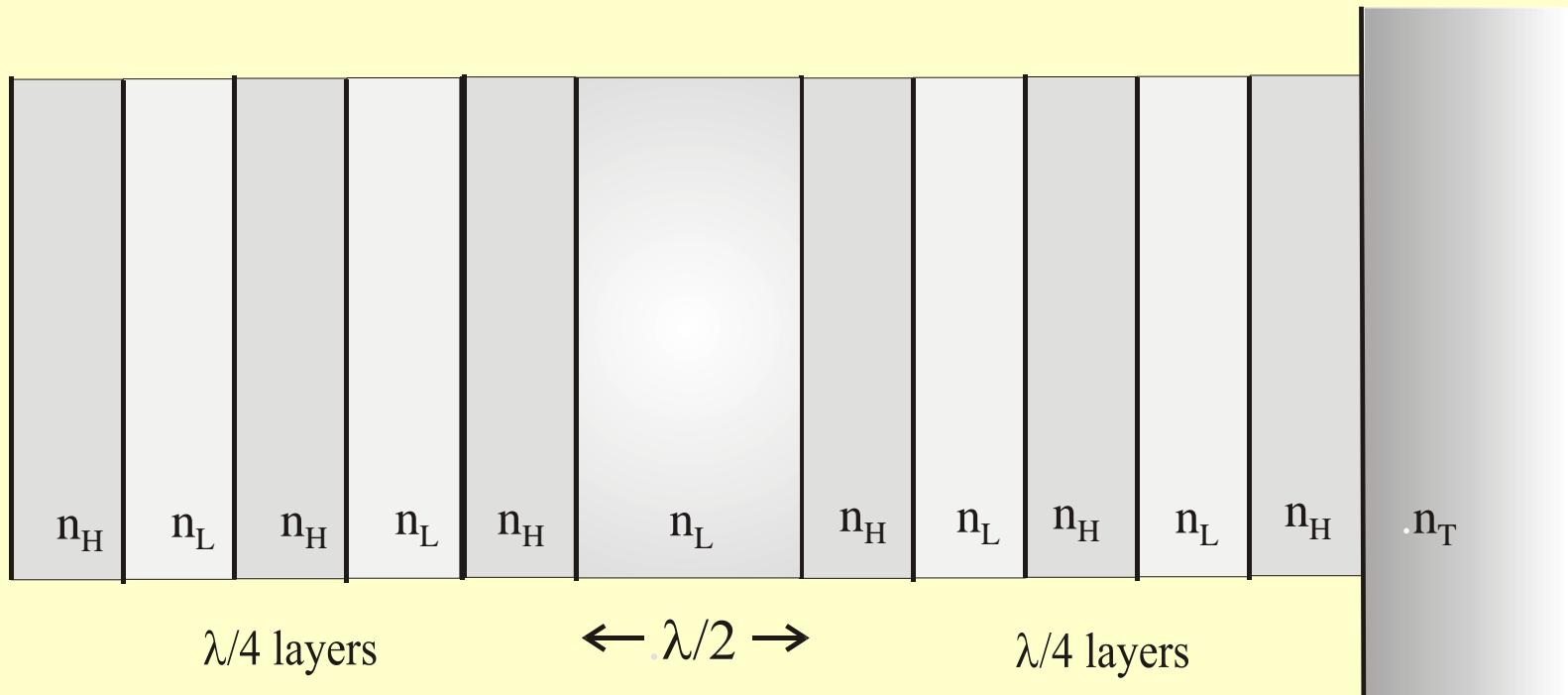
*Interference filter; composed of multi-layer stacks*
