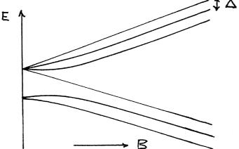
20. The diagram shows the hyperfine structure of the ground level of one of the isotopes of hydrogen, as a function of an applied magnetic field *B*. Make a rough copy of the diagram, and label the states with appropriate quantum numbers in both weak and strong fields. What is meant by a "strong" field in the context of hyperfine structure?
