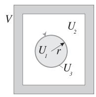
A composite system in a chamber of fixed volume V. The system comprises a rubber balloon and two fluids: one inside and one outside the balloon.
