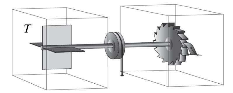
Exploit thermal fluctuations to raise the load. Seems to allow violation of Kelvin statement?
