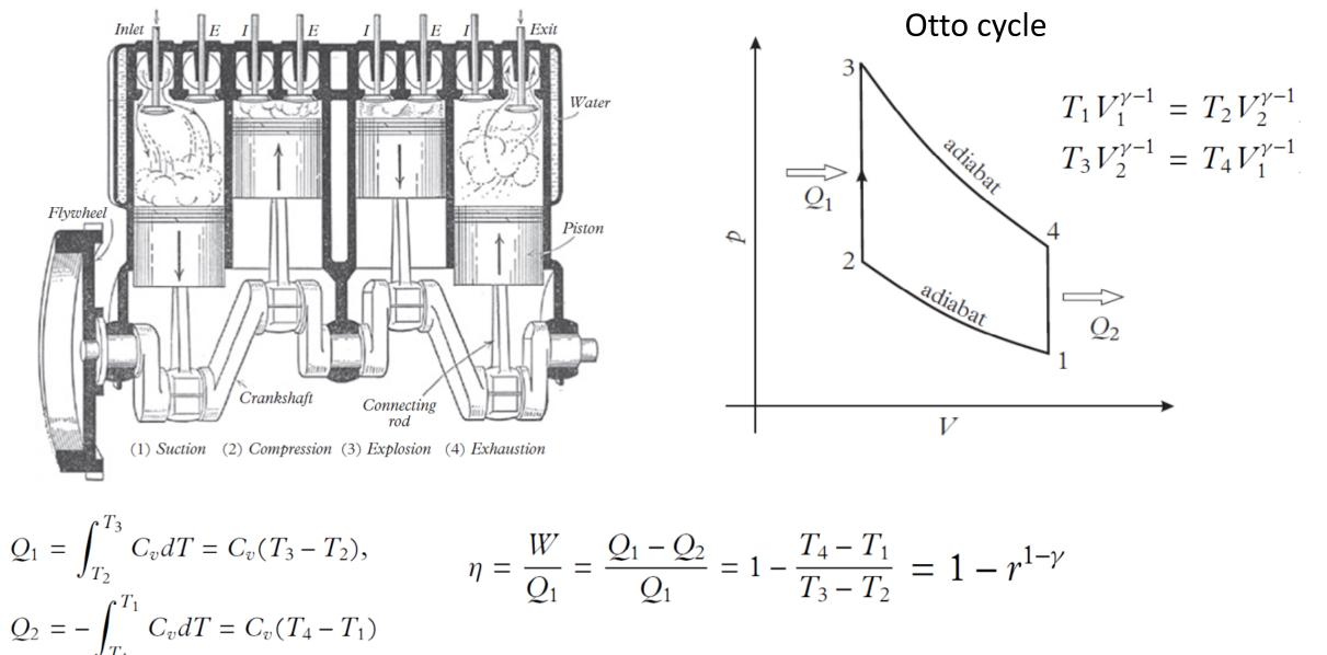
$r \equiv V_1/V_2$  is the compression ratio
