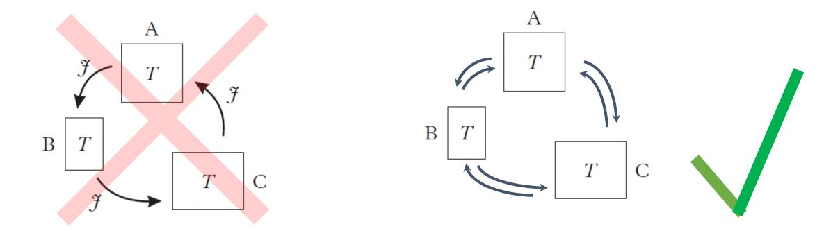
Each internal process goes at the same rate as the direct reverse process between the same two states.
