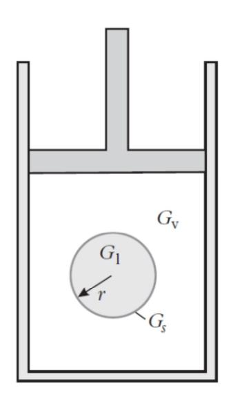
A spherical drop of liquid forming inside a vapour
