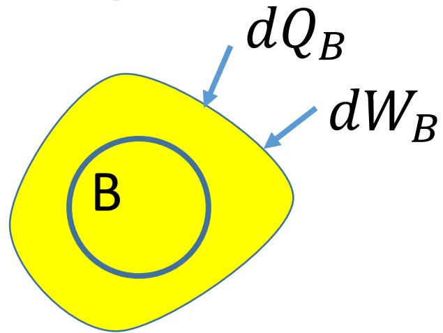
$$\left. \begin{aligned} \oint \frac{dQ_A}{T_A} &\leq 0 \\ \oint \frac{dQ_B}{T_B} &\leq 0 \end{aligned} \right\} \text{ for any processes } A, B.$$
