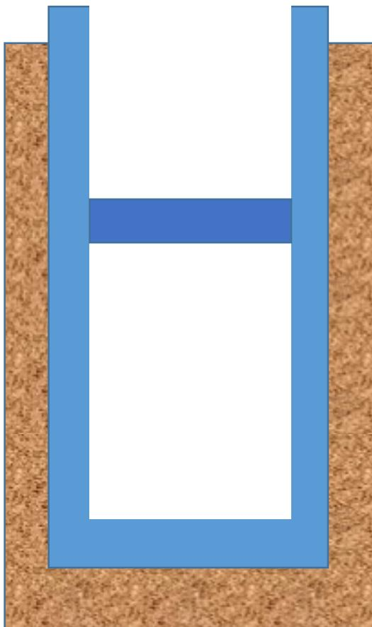
2. Thermally isolate the fluid and have it expand some more (so the fluid cools down).
