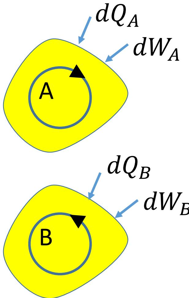
$$\left. \begin{aligned} \oint \frac{dQ_A}{T_A} &\leq 0 \\ \oint \frac{dQ_B}{T_B} &\leq 0 \end{aligned} \right\} \text{ for any processes } A, B.$$
