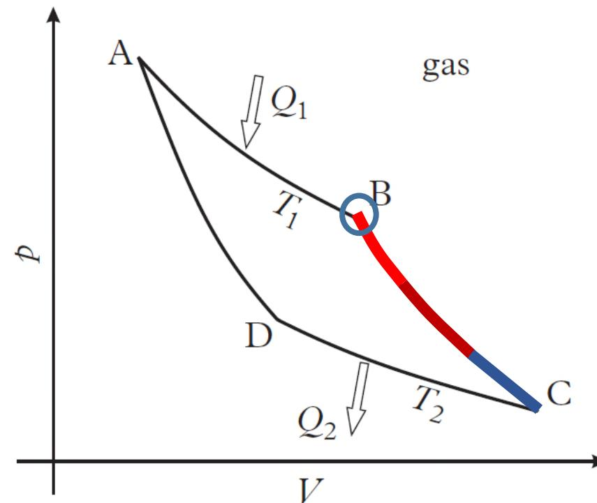
3. Contact the container with a cold reservoir and compress the fluid (the reservoir keeps it cool).
