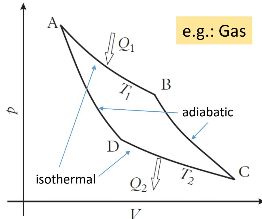
1. Thermal contact between the container and hot reservoir;
