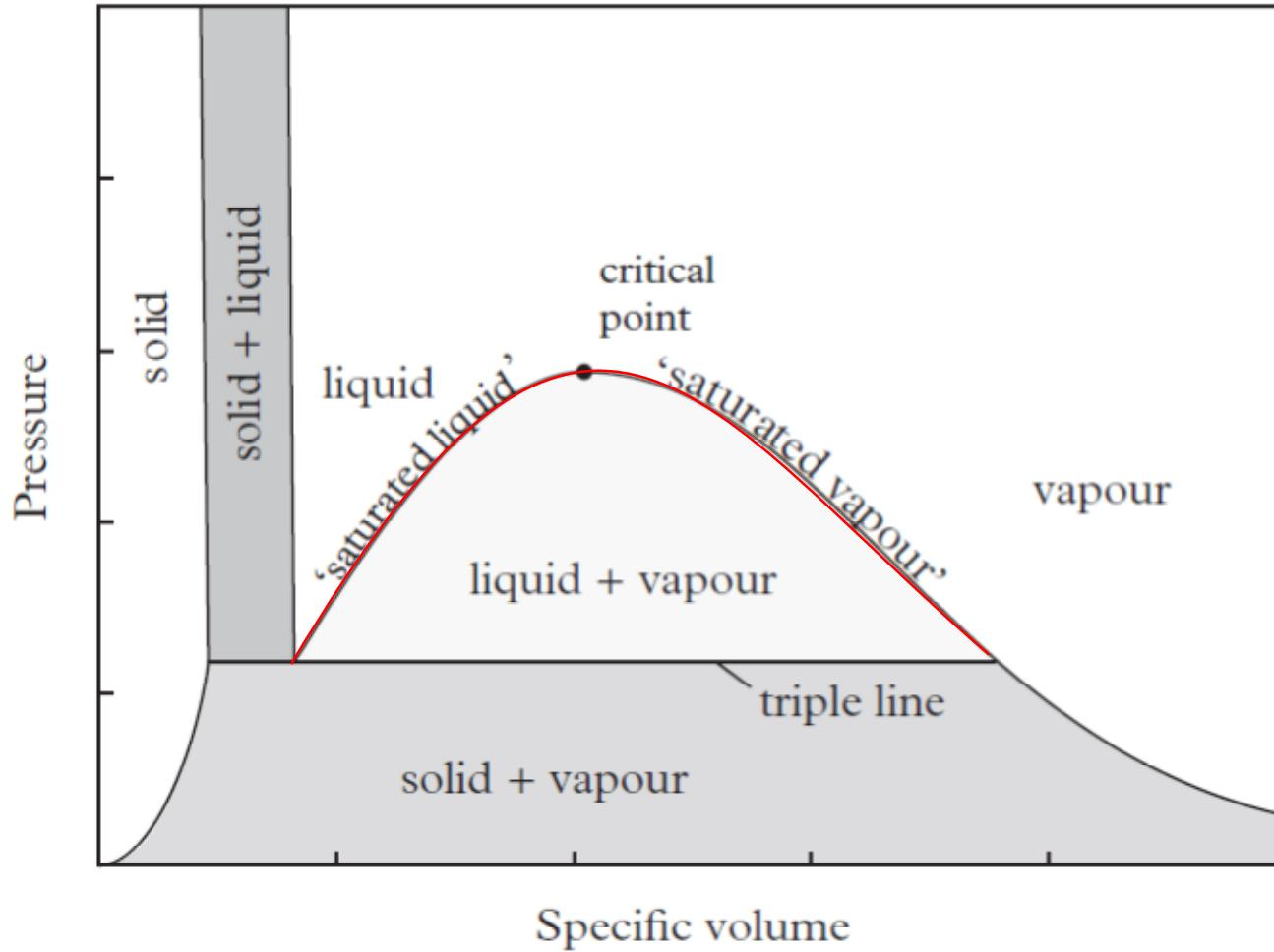
A vapour which would begin to condense if the temperature were lowered is called "**saturated**".
