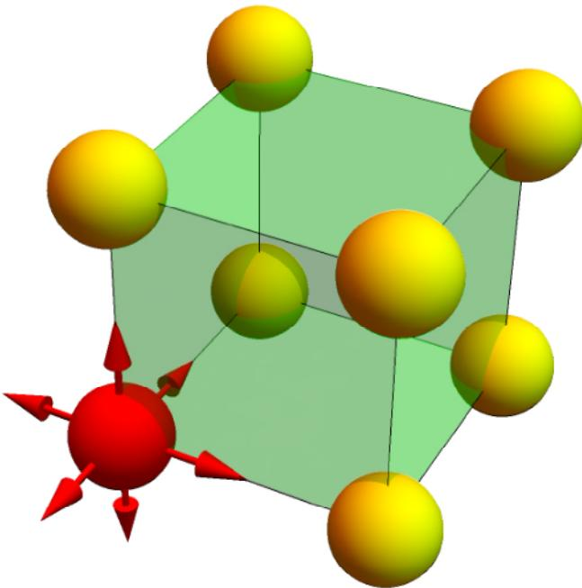
Diagram to illustrate the idea of an atom in a crystal vibrating around its equilibrium position. (Of course, all the atoms vibrate in practice, not just one!)
