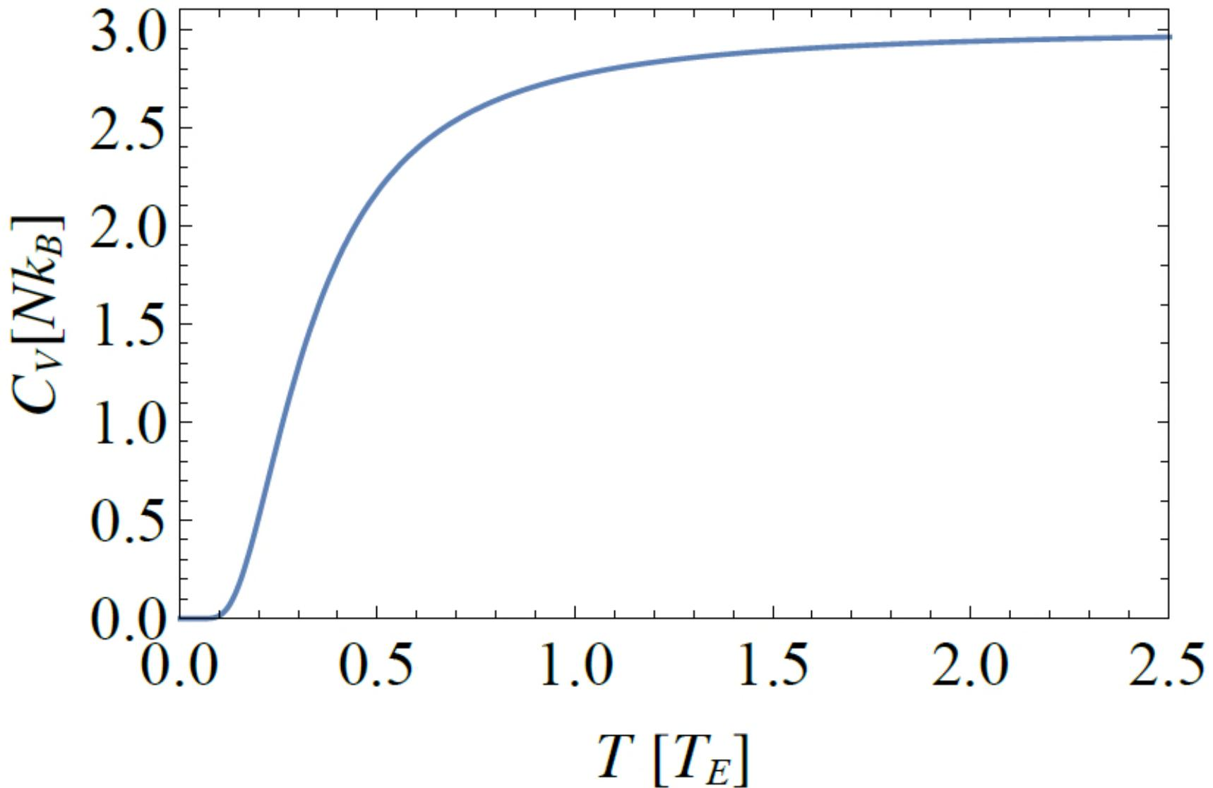
Heat capacity of a 3-dimensional crystal owing to vibrations, according to a simple model (the Einstein model) which only allows for one vibrational frequency.
