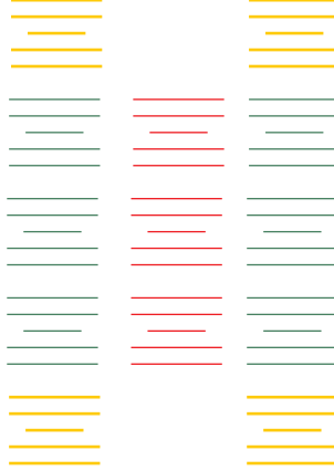
Fig. 5. Physical layout for a computer based on a two-layer concatenated code. Each horizontal line represents a block of 23 qubits encoded in the inner code. A group of 5 such lines replaces each bit in fig. 3. A single data block with a pair of ancillas is shown.
