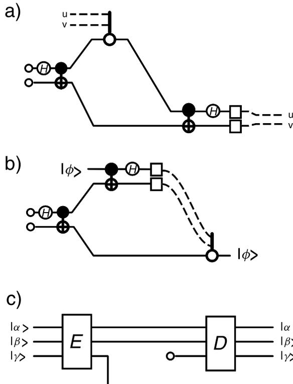
**Figure 9.** Basic quantum communication concepts. The figure gives quantum networks for (a) dense coding, (b) teleportation and (c) data compression. The spatial separation of Alice and Bob is in the vertical direction; time evolves from left to right in these diagrams. The small boxes represent measurements, the broken curves represent classical information.
