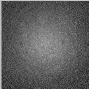
TOF image of fermionic band insulator after sudden release
