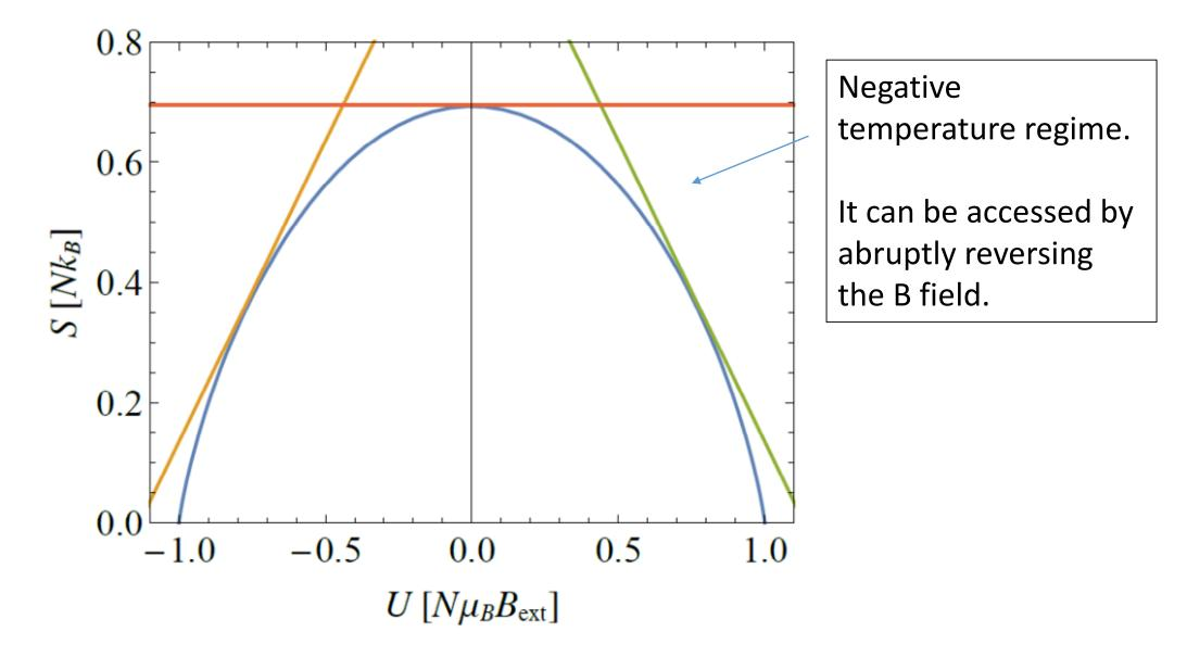
The straight lines give three examples of the slope (dS/dU).
