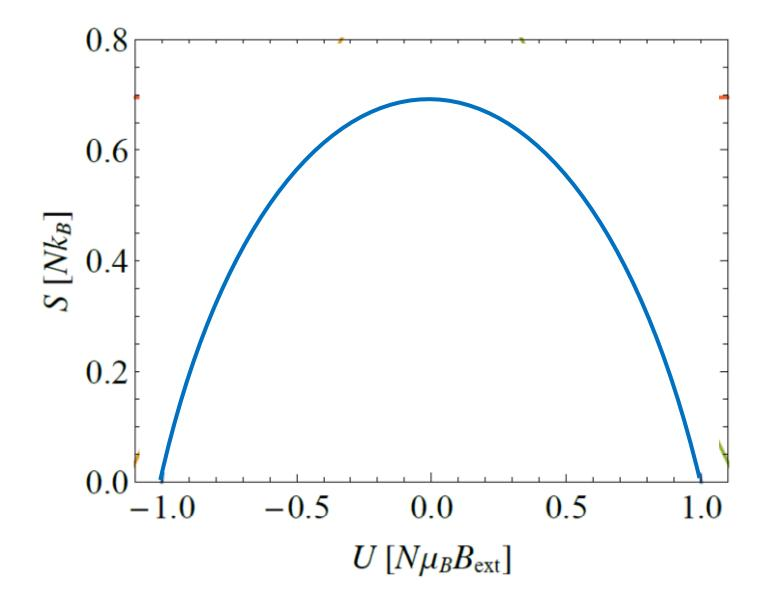
Entropy of a paramagnet as a function of internal energy.
